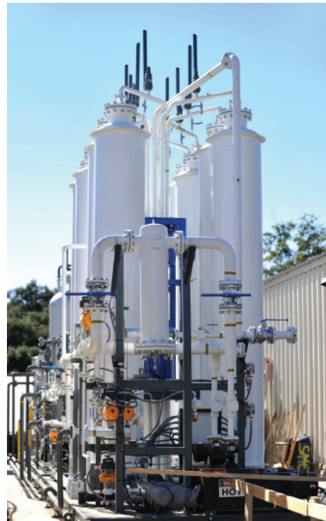
ESCONDIDO ENERGY: A project in Escondido, Calif., which is in the testing stage, aims to process biogas into natural gas and inject it into the pipeline.
