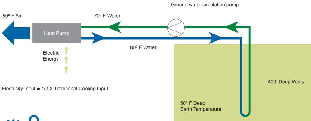
Electricity Input = 1/2 X Traditional Cooling Input
