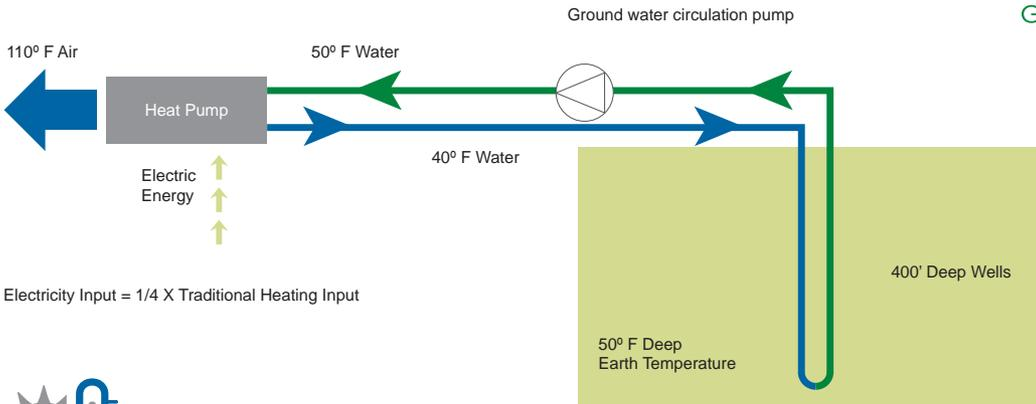
Electricity Input = 1/4 X Traditional Heating Input
